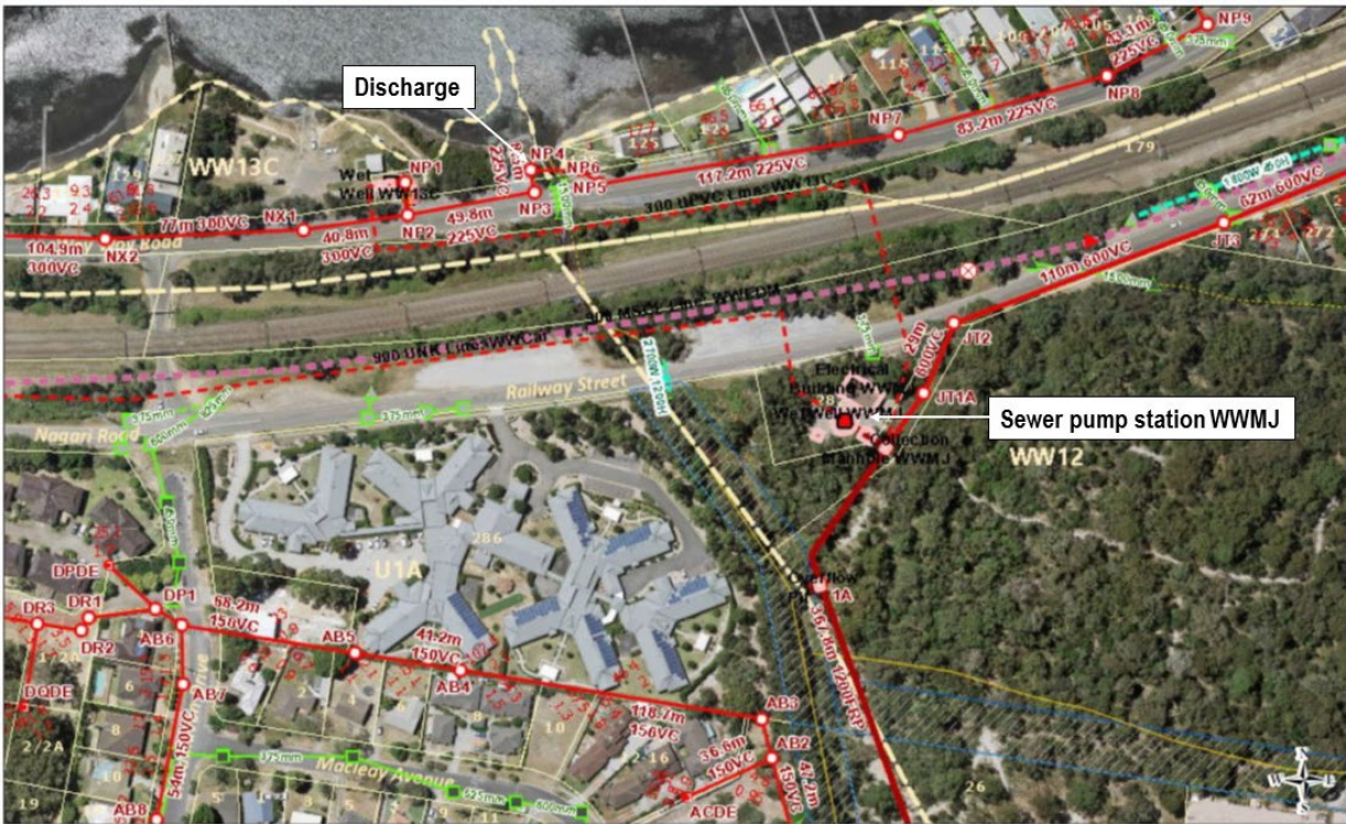
Figure 13: Sewer pump station WWMJ and discharge
